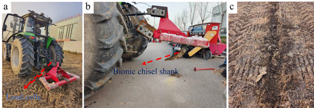
Figure 6. Measurement of draft force for the bioinspired subsoiler: (a) experimental setup; (b) soil-tool adhesion phenomena of the wet soil; (c) resulting furrow profile.
