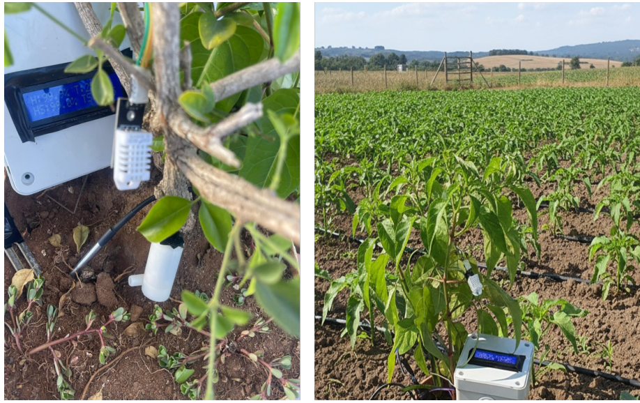
Figure 4. Deployment of our IoT measurement unit in an agricultural field for validation.
