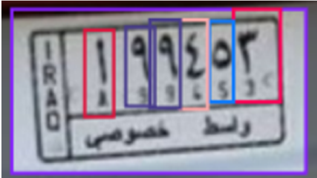
Figure 4.2. A licence plate example using single-character detection
