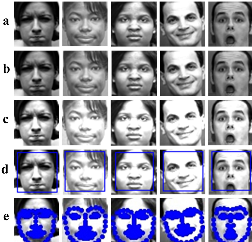
Figure 4. sample images of a human face with an emotion (a) input images (b) noise removed images (c) contrast-enhanced images (d) face detected images (e) landmark extracted images.
